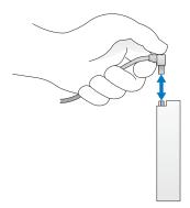
When connecting an IDE cable, ensure you align the colored stripe with the pin 1 connector. When disconnecting an IDE cable, grasp the colored pull tab and pull until the connector detaches.
